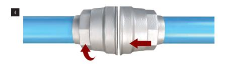
4. Only for tube diameters D50 and D63mm. To facilitate installation, fittings are supplied with unscrewed nuts. Once the tube is inserted into the fitting, tighten the nuts to the torque specified below.
